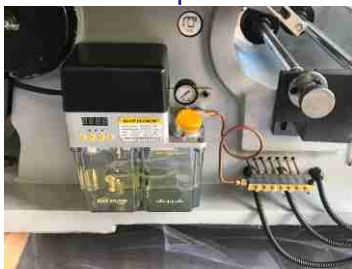
automatic oil system
